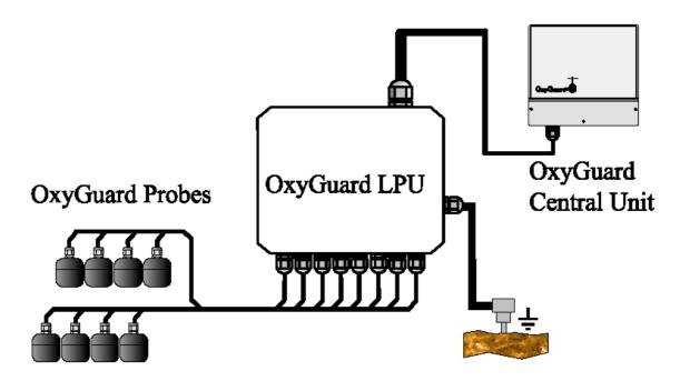
The OxyGuard Lightning Protection Unit is a surge suppressor that will prohibit transient surges in the probe leads from damaging transmitters in the central unit.
